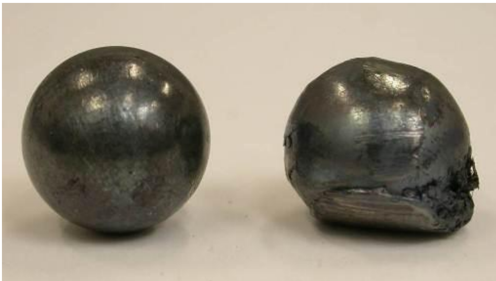
Figure 7 - Reference ball and ball with friction damage (Photo: Exova)
