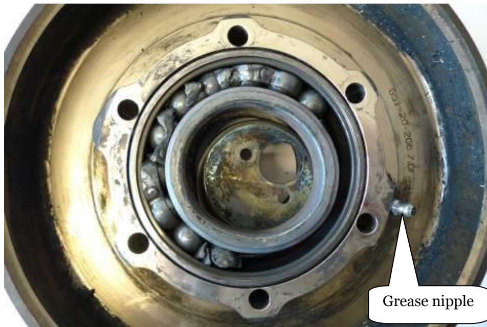
Figure 6 - The pulley mounted on the engine; note that the ball bearing's inner bearing race is elliptic. The bearing's ten balls have been compressed in a part of the bearing. The ball cage has been damaged, allowing the balls to move so that the distance between the balls is not evenly distributed.
