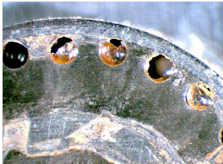
Photograph 6. Part of the injection nozzle showing foreign material
