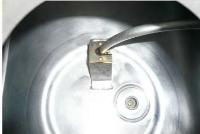
Photo 1 Area to be inspected as seen from top of the fuel tank with Fuel level sensor P/N SA 210-08095-01 removed
