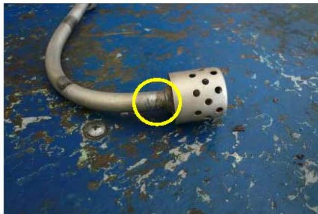
Photo 2 Example of signs of damage on Fuel suction tube assembly P/N SA202-18112-07
